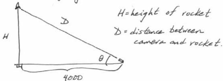
$$\text{speed} = \frac{\text{change in height}}{\text{as time changes}} = \frac{dH}{dt} \quad (2)$$
